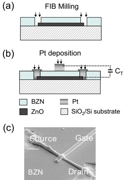
FIG. 2. (Color online) Scheme of the fabrication processing for top-gated ZnO NW FET with BZN dielectric. (a) Ion beam was focused at both ends of the individual ZnO NW to mill away the BZN layers and uncover the clean ZnO NW surface. (b) Pt is deposited onto both ends of the exposed ZnO NW and across the middle of the ZnO NW, thus forming the source, drain, and gate electrodes. (c) SEM image of the fabricated top-gated ZnO NWT with BZN dielectric.
