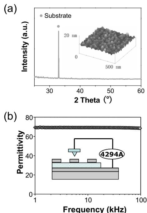
FIG. 1. (Color online) Characteristics of BZN dielectric layer. (a) XRD pattern of the BZN film and AFM image of the as-deposited BZN film (inset). (b) Permittivity as a function of frequency for the amorphous BZN film, measured without dc bias field. Inset is the Pt/BZN/Pt/ $\text{SiO}_2/\text{Si}$  paralleled structure for capacitance measurement.
