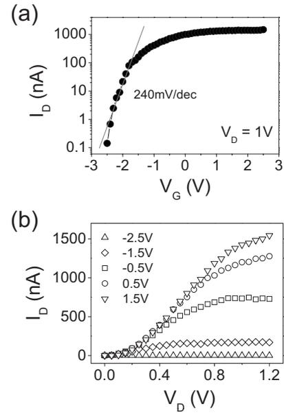
FIG. 3. Electric transport measurements. (a)  $I_D$ - $V_G$  transfer characteristics of the ZnO NW FET with BZN top gate. (b) Curves of current vs source-drain bias under various gate voltages.
