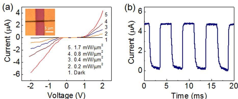
FIG. 2. (a)  $I$ - $V$  Curves of CdSe nanowire under light illumination with varying intensities. The inset shows the optical microscopic image of single CdSe nanowire electrical device. (b) Photoresponse time of the nanowire device under a 200 Hz square wave modulated light illumination. The light intensity is 1.7  $\text{mW}/\mu\text{m}^2$ , and the bias voltage is 2 V. It shows a photocurrent response time less than 300  $\mu\text{s}$ .
