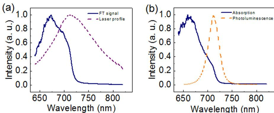
FIG. 3. (a) Direct FT spectrum of frequency encoded CdSe nanowire photocurrent (solid line) and the supercontinuum laser spectrum (dashed line); (b) Normalized FT spectrum by the laser spectrum, i.e., absorption spectrum of CdSe nanowire (solid line). The dashed line shows photoluminescence spectrum of the same CdSe nanowire. The bandgap was determined to be 1.75 eV by the cutoff wavelength in the absorption spectrum, which is consistent with the peak wavelength of photoluminescence.
