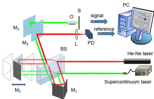
FIG. 1. Experimental scheme of supercontinuum laser based Fourier transform spectrometer for absorption measurement of quasi-one-dimensional individual nanomaterial. BS, beam splitter; M, mirror; O, objective; S, sample; L, lens; PD, silicon photodiode.
