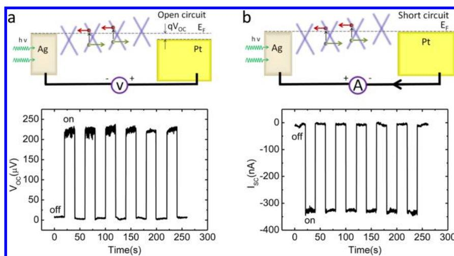
**Figure 2.** Performances of vertical Ag–SFLG–Pt device. The photoelectrical properties were measured under laser irradiation with 514 nm wavelength. (a) The mechanisms of the photogenerated open-circuit voltage ( $V_{OC}$ , upper panel) and the  $V_{OC}$  outputs under on–off light modulation (lower panel). (b) The mechanisms of the photogenerated short-circuit current ( $I_{SC}$ , upper panel) and the  $I_{SC}$  outputs under on–off light modulation (lower panel).
