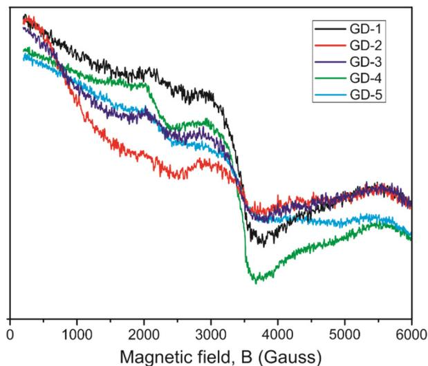
**Fig. 13.** EPR spectra of five rock varnish samples. Signals of Mn(IV) occur at ~3300 G.
