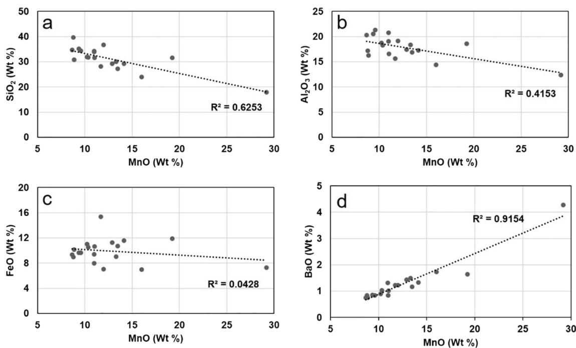
Fig. 8. Correlation curves of elements with Mn. Mn content shows a negative correlation with Si (a) and Al (b) and a positive correlation with Ba (d). Fe content does not change as a function of Mn (c).
