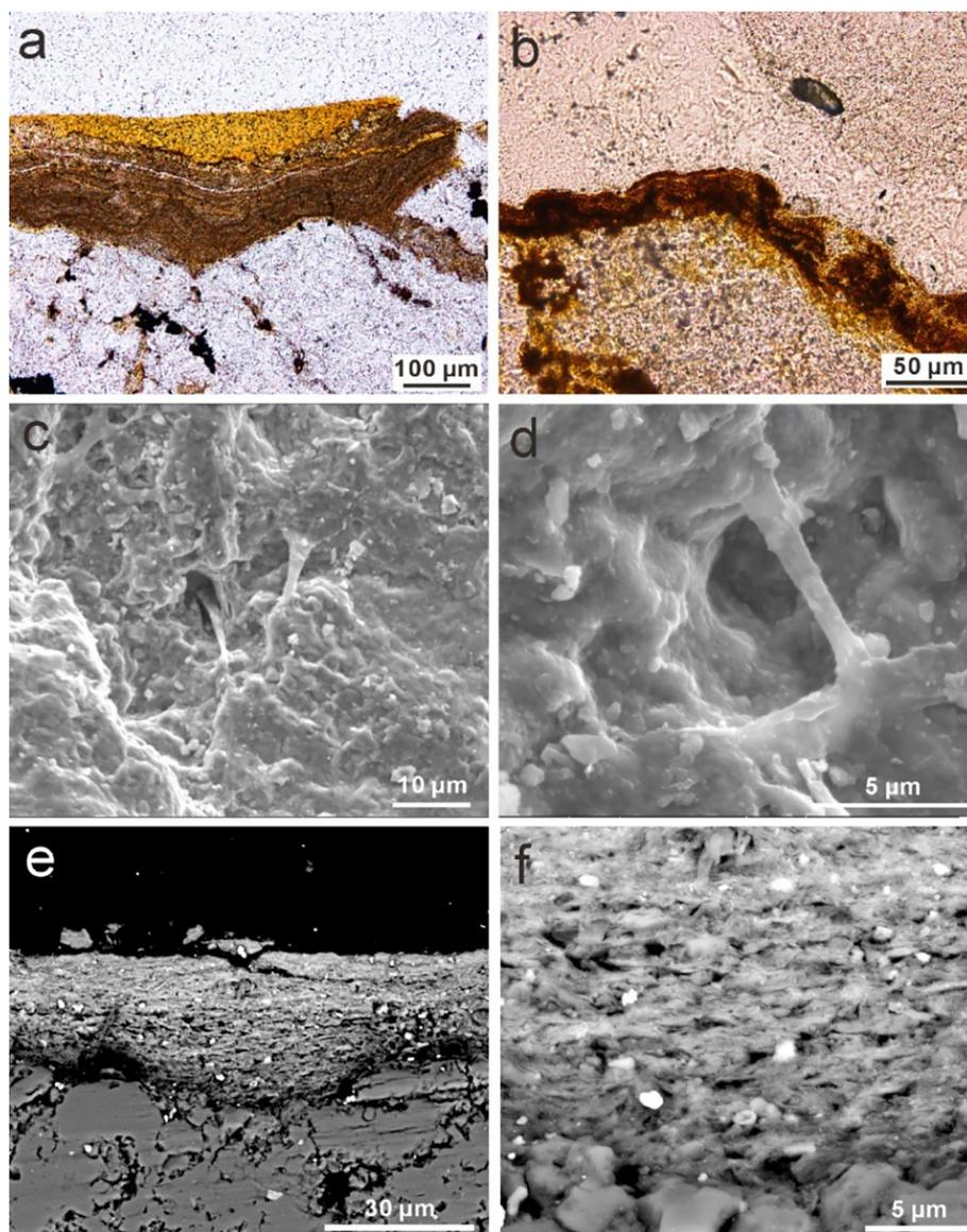
**Fig. 2.** Morphology of rock varnish under OP (a–b) and SEM (c–f). (a) (b) Layered varnish with alternating microlaminations. (c) (d) Secondary electron images demonstrating cave structures on the varnish surface. (e) (f) Back-scattered images showing fine mineral grains and small tunnels on the sample cross profile. Fig. 2b is revised from our previous work Lu et al. (2019).
