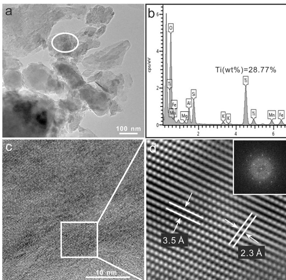
Fig. 7. TEM morphology (a), EDS data (b), lattice photograph (c, d) and diffraction pattern (d) of Ti-rich grains. Panel b shows the chemical composition of the selected oval area in panel a. Lattice fringes and diffraction pattern in panel d are the FFT and inverse FFT results of selected rectangular area in panel c. The  $d$  values of the two-dimensional lattices are 0.35 nm and 0.23 nm (d), and can be attributed to the crystal faces of (101) and (004) of anatase.
