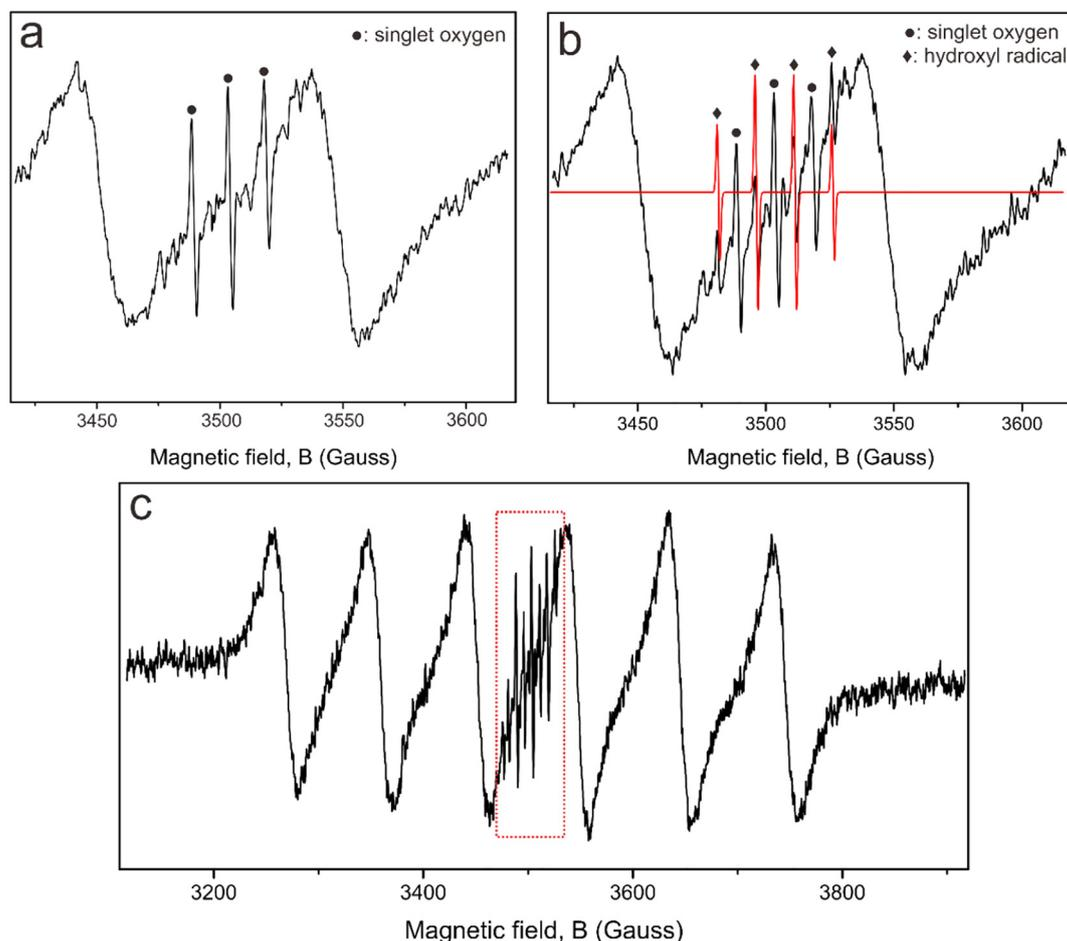
**Fig. 14.** EPR spectra of ROSs produced by varnish suspension before (a) and after illumination (b, c). Panel b is the magnified version of the red rectangle region in panel c. The red curve in panel b is the standard signals of hydroxyl radical. (For interpretation of the references to color in this figure legend, the reader is referred to the web version of this article.)
