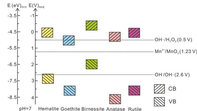
Fig. 16. Diagram of band edge position of semiconducting minerals in rock varnish. Dash lines indicate the redox potential of some half reactions (Pelizzetti and Minero, 1993; Sherman, 2005).
