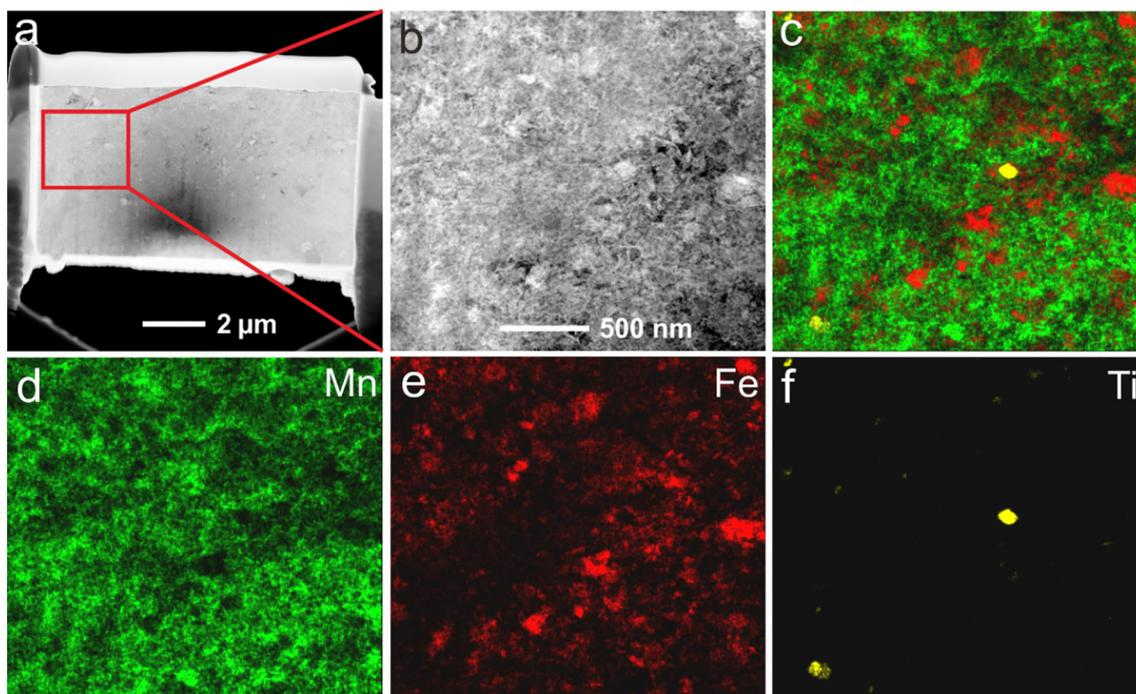
**Fig. 12.** Element distribution maps obtained by STEM. Panels a and b are overview images. Panel c is an overlay of Mn (green), Fe (red) and Ti (yellow) distribution. Most of the black areas in this panel are rich in Si. Panels d, e and f are a Fe map, Mn map and Ti map, respectively. (For interpretation of the references to color in this figure legend, the reader is referred to the web version of this article.)
