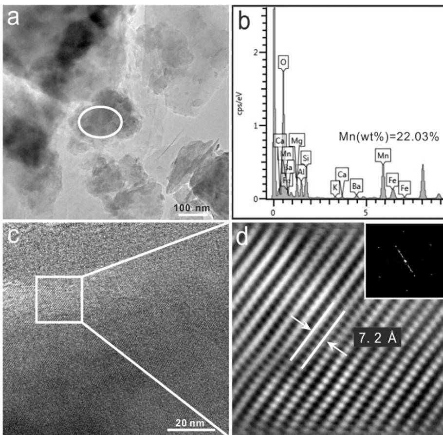
Fig. 5. TEM morphology (a), EDS data (b), lattice photograph (c, d) and diffraction pattern (d) of Mn-rich grains. Panel b shows the chemical composition of the selected oval area in panel a. Lattice fringes and diffraction pattern in panel d are the FFT and inverse FFT results of selected rectangular area in panel c. The  $d$  value of the one-dimensional lattices is 0.72 nm (d) and can be attributed to the crystal faces of (001) of birnessite.
