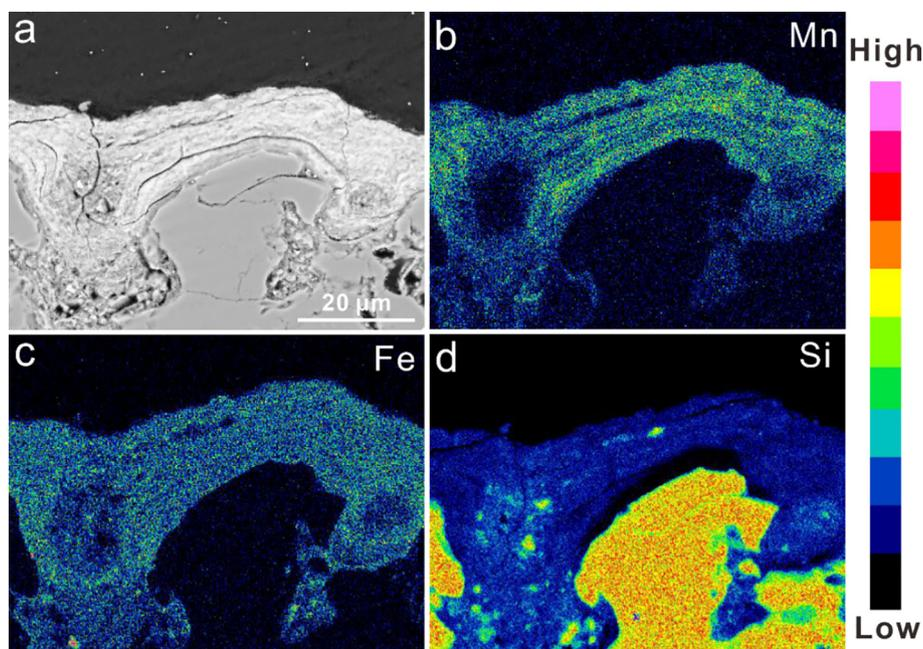
Fig. 11. EDS mapping of elements within varnish thin section under SEM. This figure is revised from our previous work Lu et al. (2019).
