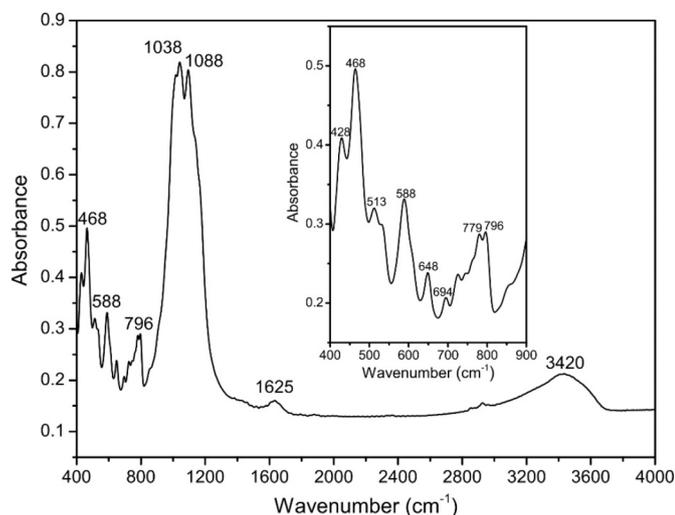
Fig. 3. FTIR spectra of rock varnish powders. The signals in the range of 400–900  $\text{cm}^{-1}$  are magnified in the inserted rectangular region.
