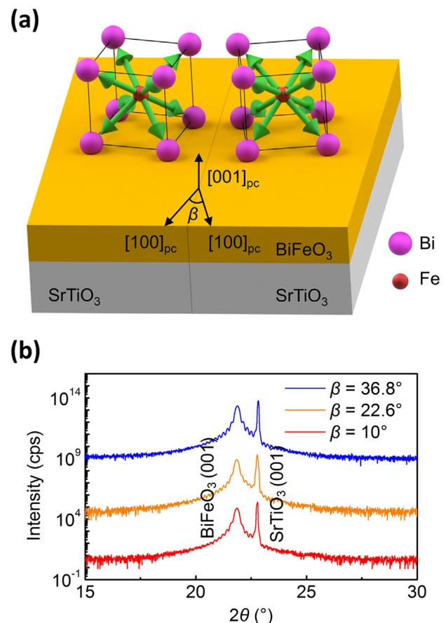
**Fig. 1.** (Color online) BiFeO<sub>3</sub> bicrystal thin film. (a) Schematic diagram of epitaxial BiFeO<sub>3</sub> thin films grown on SrTiO<sub>3</sub> bicrystal substrates. BiFeO<sub>3</sub> have eight possible polarization orientations. (b) XRD profiles of BiFeO<sub>3</sub>/SrTiO<sub>3</sub> heterostructures revealing the highly crystalline quality of BiFeO<sub>3</sub> thin films.
